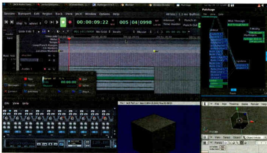
Ubuntu Studio 9.10 is shown multitasking with JACK Audio Connection Kit: Qt Interface 0.3.4, Ardour 2.8.2, Patchage 0.2.3, Hydrogen 0.9.3, Blender 4.29a.
