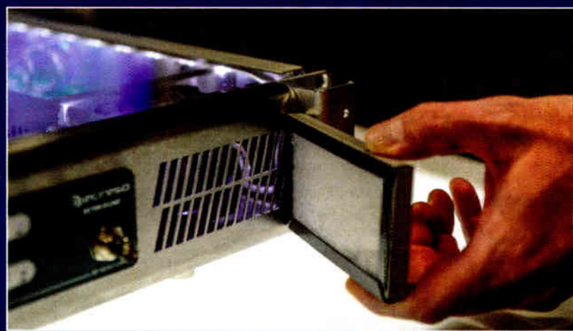
A magnetic mount makes it easier to change filter media on this Egreso product.
