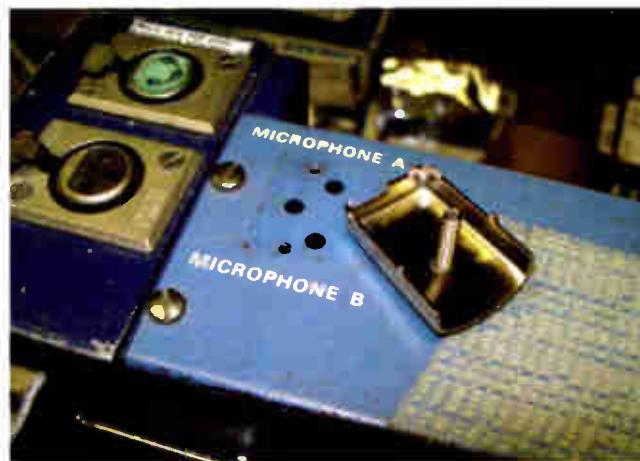
Fig. 3: The new handle uses a single #6 screw attachment on each end.
