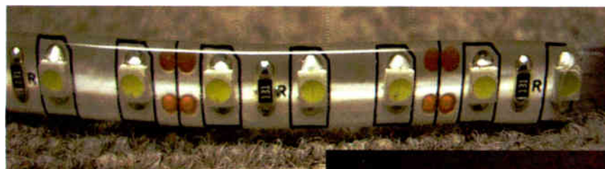
Fig. 1: A closeup of the LED strip, with built-in dropping resistor.
