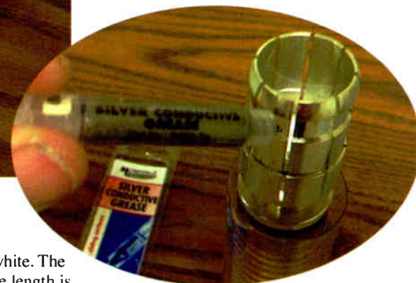
Fig. 4: Improve bullet conductivity using MG Chemicals' silver grease.
