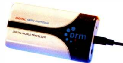
Fig. 5: The Coding Technologies Digital World Traveller was a convenient shortwave accessory for the traveler with a PC on the go.
