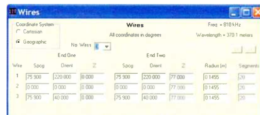
Fig. 1: Array geometry moment method model for three-tower in-line array.
