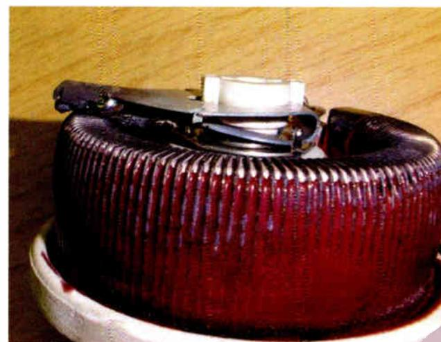
Fig. 4: The repaired rheostat with its solder blob contact.
