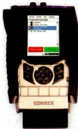
ACCESS Portable lets you send studio-quality live audio, real time over IP using 3G, 4G, Wi Fi, BGAN/VSAT, PSTN or DSL to make any remote broadcast really stand out. Connect with your audience from anywhere, live, with the easy to use, handheld ACCESS Portable!
