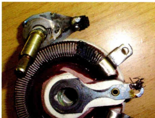
Fig. 3: Disassemble to repair the bad contact.
