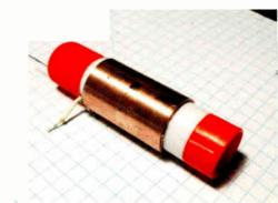
Fig. 9: The finished piston capacitor.
