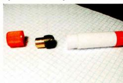
Fig. 6: Add a short piece of copper tubing to the glue well (black plastic) of the movable piston.
