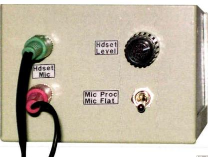
Mics in these units are DC powered and the computer typically supplies 5 volts (unloaded). The tiny load that is the mic's FET amplifier drops the voltage to about 2.5 volts, and the voltage variation around this axis point is the actual audio from the mic. Most computers use an internal series resistor of about 10 k-ohms; that's what we've used as well.
