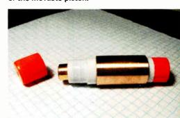
Fig. 7: Add the outer copper tubing, which forms the other capacitor plate.
