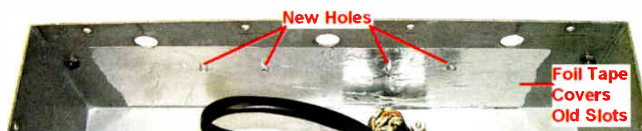
Fig. 4: Inside the case with the foil tape covering the openings.
