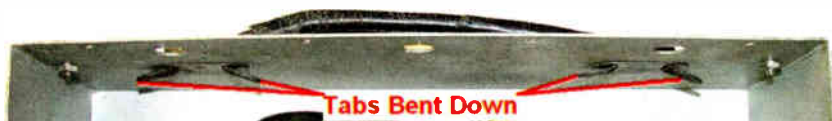
Fig. 2: Begin by bending the tabs away from the inside of the cabinet.
