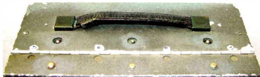
Fig. 1: The original leather handle on a WX-2A meter.
