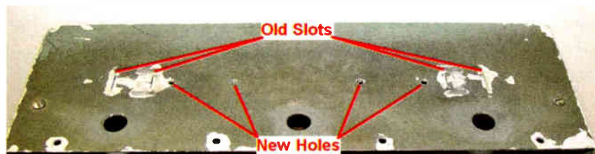
Fig. 3: The original handle is gone and new holes are drilled.
