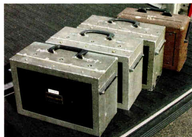
Fig. 6: From left to right, an RCA WX-2A, an RCA WX-2C, an RCA WX-2D, all with new handles, and a stock Potomac Instruments FIM-41.
