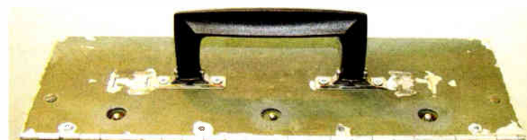
Fig. 5: Here's the meter with its new hinged handle standing proud.
