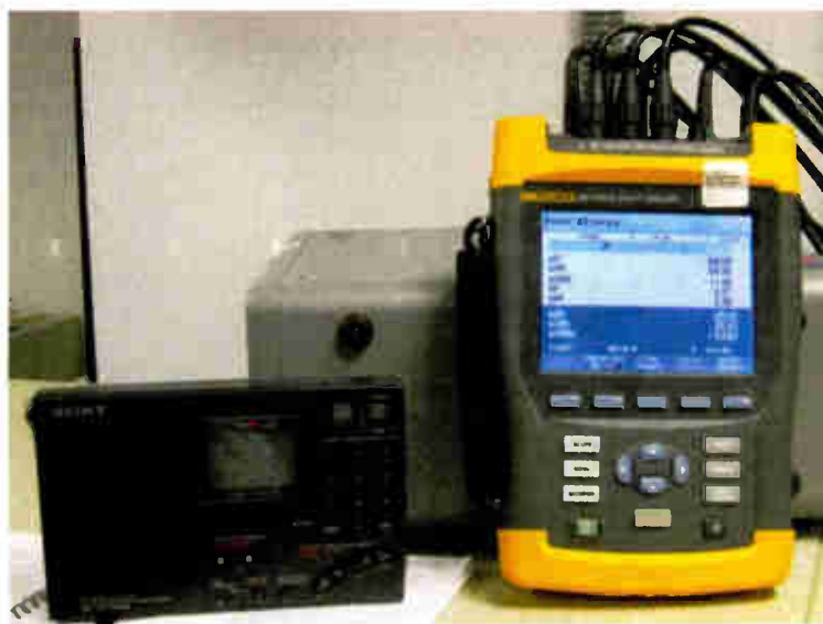
The Fluke 434 power quality analyzer was used to measure the actual total AC power consumption of the transmitter with and without MDCL applied. The Sony ICF-SW7600 portable receiver was one of the receivers used to check for audio quality and coverage with the MDCL switched on and off.
