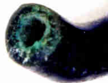
Fig. 2: Corrosion can migrate along insulated wire, rendering it useless.
