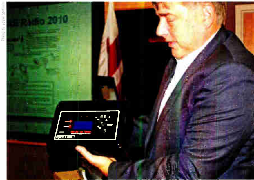
NPR Labs' Rich Rarey holds the first PAIS-enabled HD Radio receiver. Created at NPR Labs and based on iBiquity's 1281/1282 reference receiver, the unit has 96 hours of internal recording time and HD Radio Conditional Access. The microcontroller code for PAIS functionality uses only 10 kB of memory. The PAIS receiver is housed in a custom enclosure with a sloping front to indicate its use as an accessible device.
