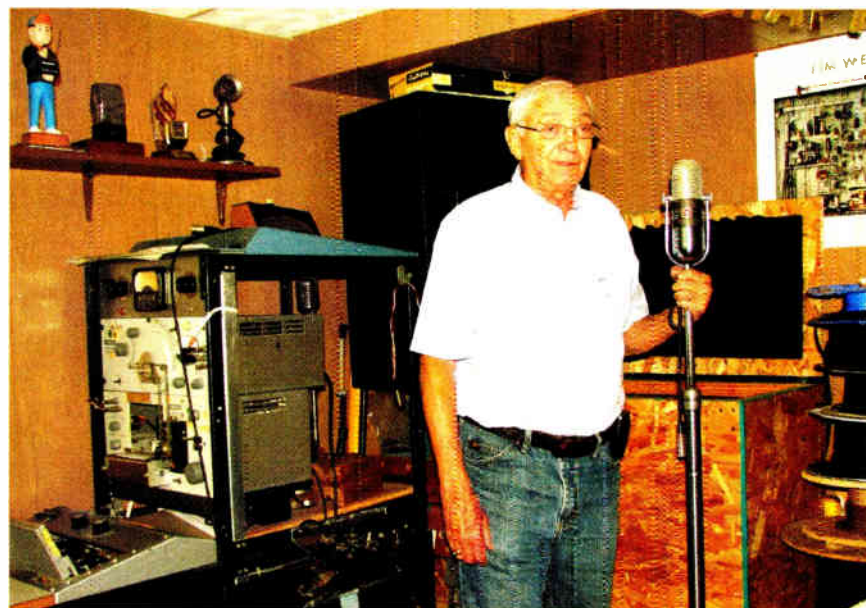
Kane with another of his ribbon mics. The device behind him is used for sweep-testing the frequency response of repaired microphones.
