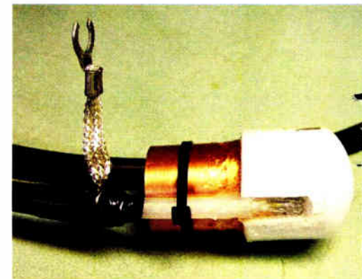
Fig. 5: Bob Meister's DIY connector adapter. Note the notch for the center conductor.
