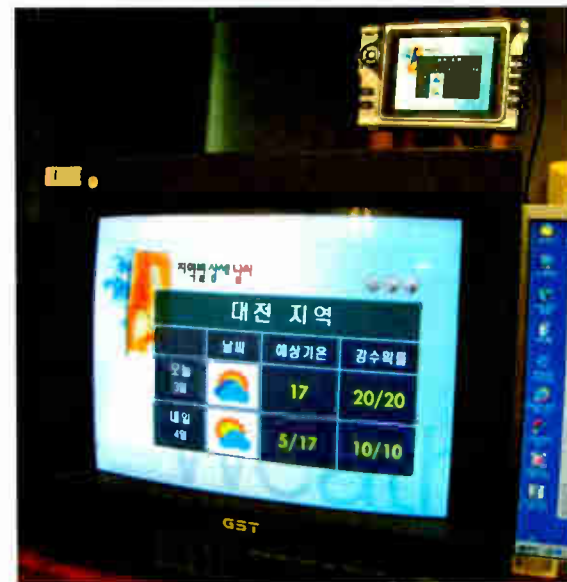
Multimedia Object Transfer Slideshow on DAB is being used by Korean radio station SBS to provide listeners weather and traffic information. The MOT protocol is part of the DAB standard.
