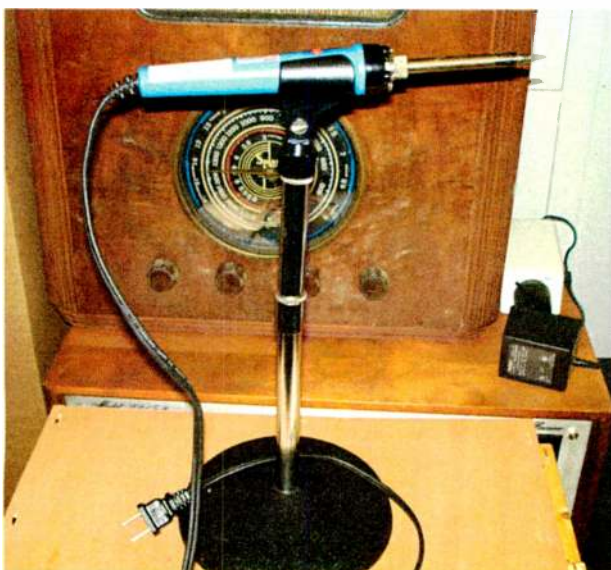
Fig. 1: A handy way to hold a hot soldering iron.
