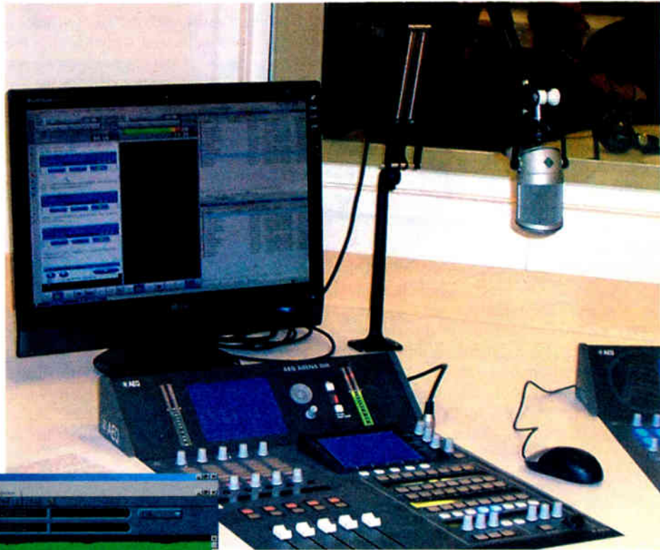
The Mar4Suite Pro can be seen on screen, above an AEQ Arena control surface, at Canarias Radio.
