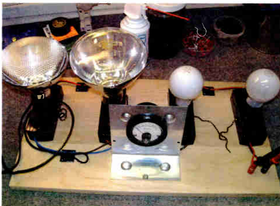
Fig. 2: A few bulbs, wood and wire make up this home-brew dummy load, used to load-test uninterruptible power supplies.
