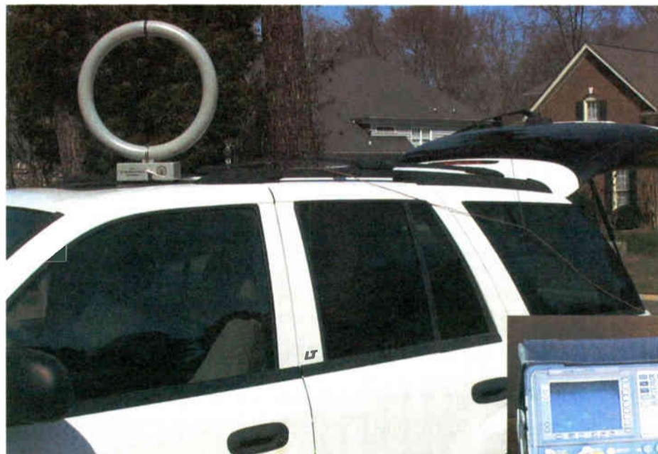
My test vehicle with loop antenna mounted on the roof. Any spectrum analyzer will work as long as it has the appropriate resolution bandwidth (300 Hz), 90 dB of dynamic range, PWR sampling and low noise specifications.
