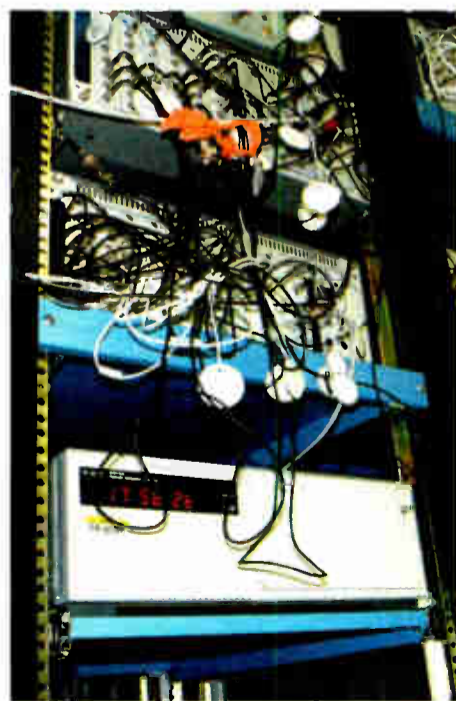
One of the five Cesium time standards and its comparator system at WWV and WWVB. The Cesium standards are all referenced to the U.S. Master Clock in nearby Boulder, and one will be taken out of service with as little as 5 nanoseconds drift.
