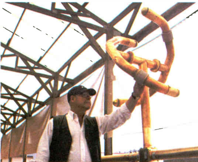
Tom Silliman with a Rototiller X Series SHPX Model Super High Power Circularly Polarized FM Antenna
