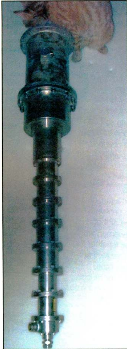
Fig. 3: Water-cooled dummy load that can be used in caloric power measurements.
