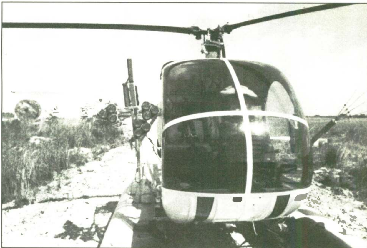
Fig. 1: Helicopter, FI meter and retro reflectors on the access road at the transmitter site.
