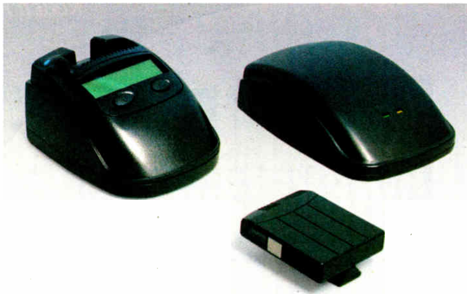
A PPM meter, hub and recharger. These innocent-looking devices are changing how radio programmers think about Arbitron data.
