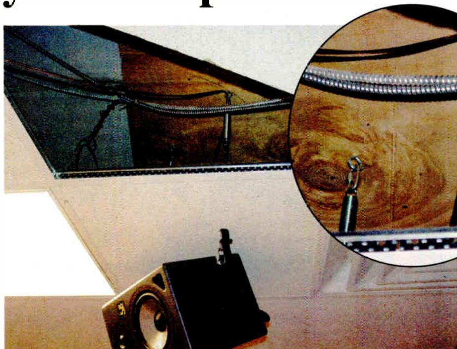
Fig. 1: You can isolate a studio speaker using springs.
