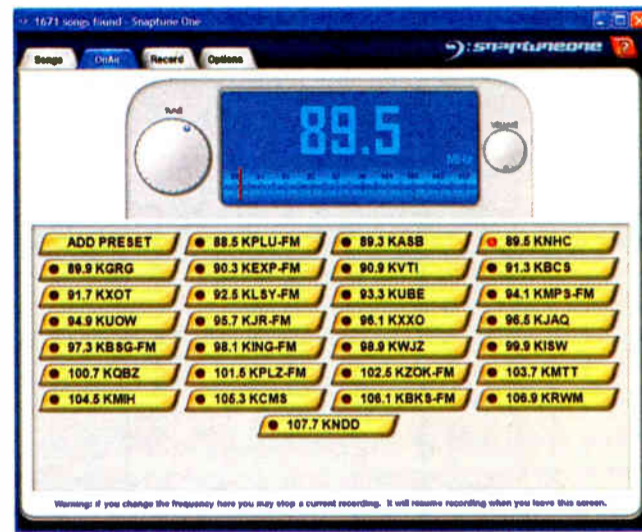
The software records songs at 64 kbps from a streamed feed of the FM station, a tuner card on the PC or a radio plugged into the PC's sound card. If the server can identify the song, it sends the information back to the user's PC and provides additional information including artist, album art and links to online retailers.
