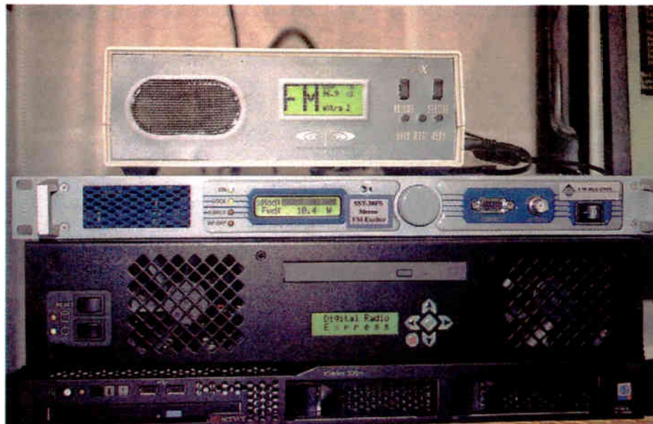
Equipment for the demo of the FMeXtra system included a DRE encoder and an Energy-Onix FM exciter feeding subcarriers into a prototype FMeXtra receiver.
