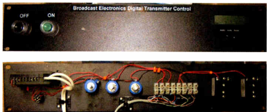
Fig. 3: A simple remote transmitter meter panel.
