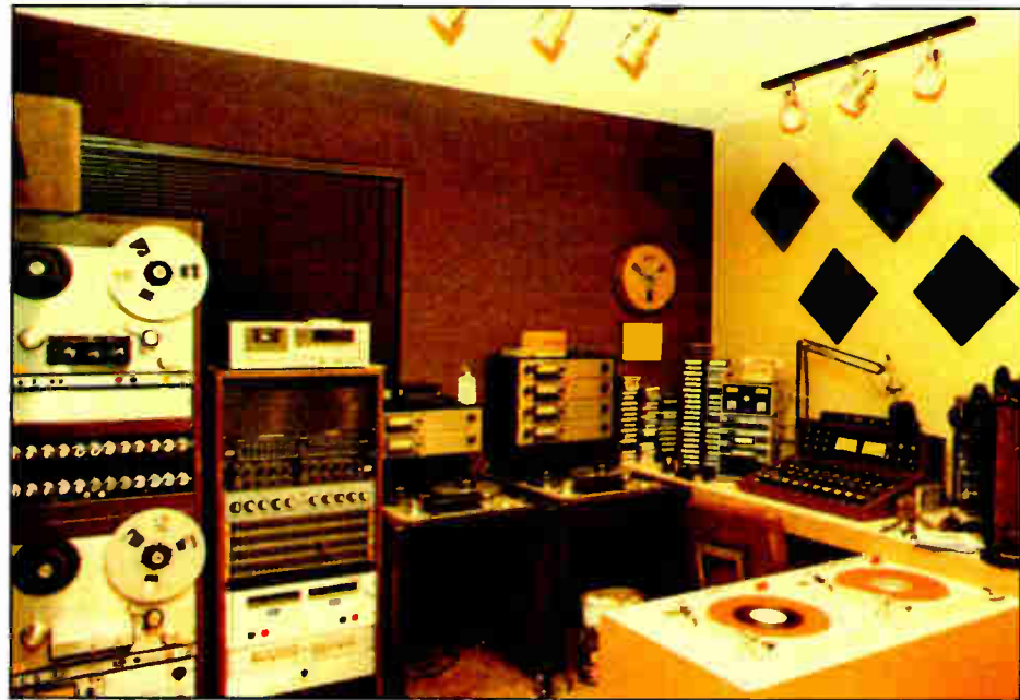
Hank Landsberg provided this photo of 'experimental' KCHZ, circa 1984. The 'Cheese-O-Mation' is the double row of knobs in the left rack. It controlled four Ampex 440 decks and a Collins TwinTape cart machine, the white unit in the short rack.
