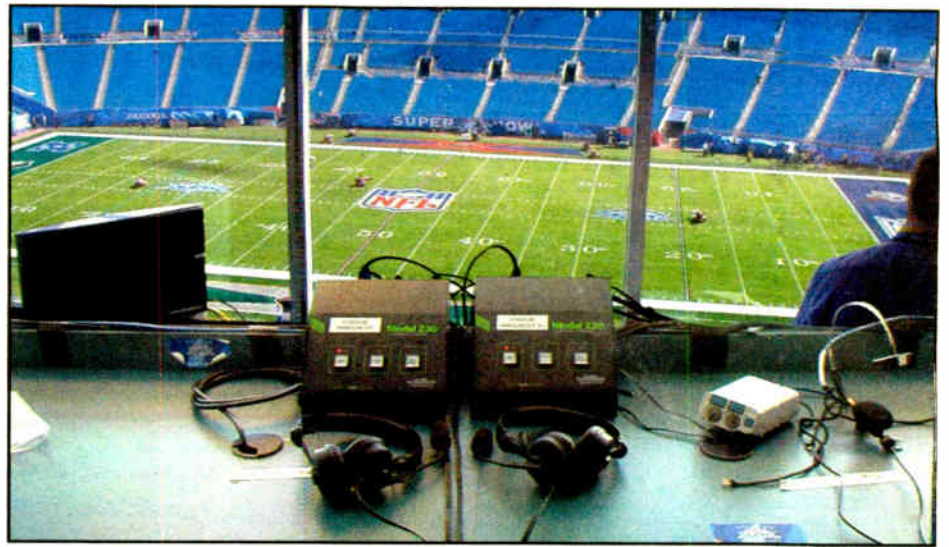
Studio Technologies Announcer's Consoles were used for Super Bowl audio coverage on CBS Radio/Westwood One as well as Fox TV .
