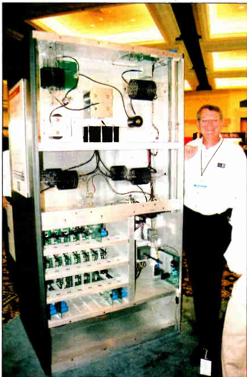
BE's Tim Bealor shows off the inside of the new 50 kW AM transmitter, the 4MX 50 AM.
