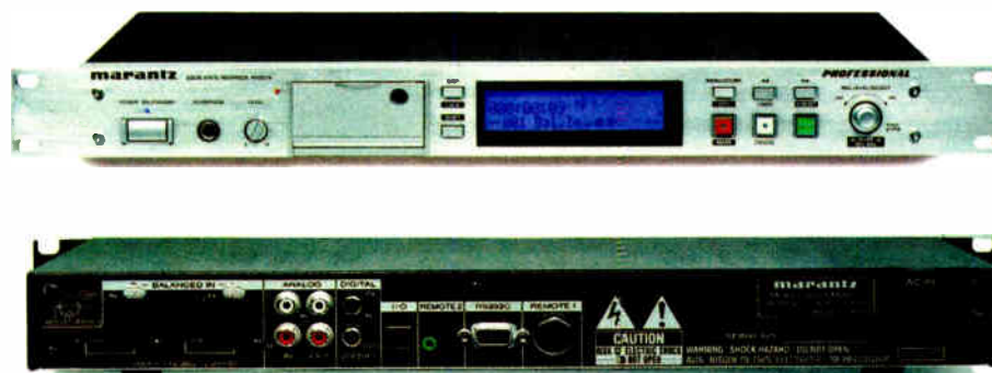
The PMD570, shown, functions like the PMD670 field recorder, but is packaged in 1 RU. Both models store audio data on Compact Flash cards.
