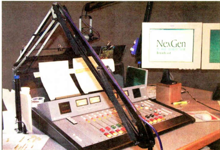
Fig. 2: 'Flocking' dampens the vibration of springs on this LPB mic arm.
