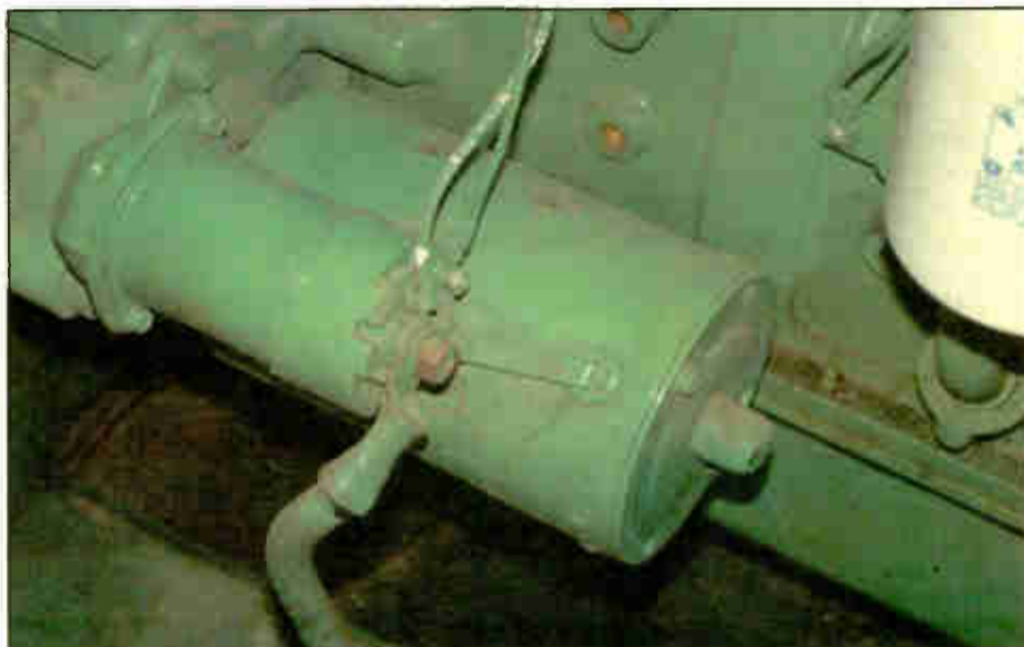
Fig. 6: A bad connection can mean an engine that will not start.
