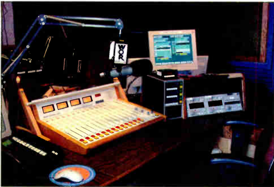
The new and the familiar in WOR's Talent Studio 2. An Audioarts board, EV RE20 mic, Denon MD and CD machines and an ITC cart machine all working with an ENCO digital delivery system.
