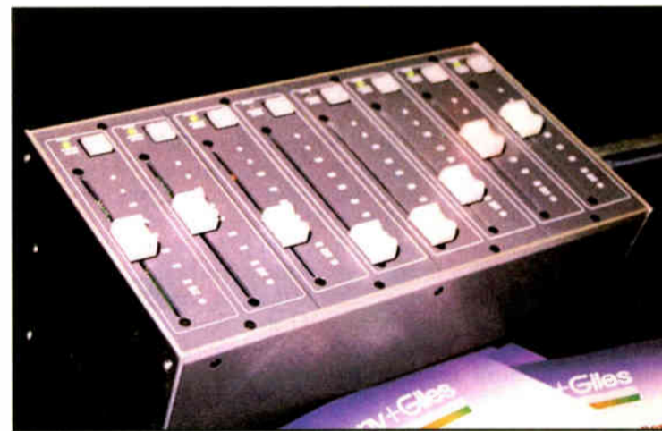
An idea looking for an application: P+G developed a fader with translucent knobs that change color based on channel status.
