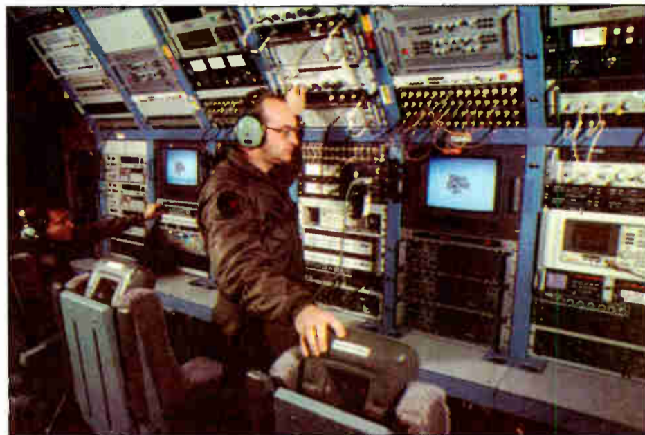
An operator verifies video quality of the aircraft's TV transmitter.
