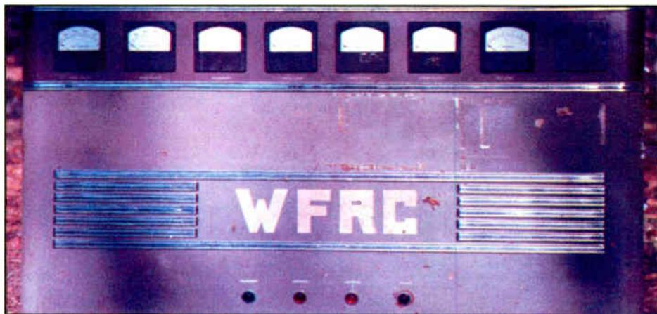
The Raytheon RA1000 was among the first to use a type of fiberglass cloth as wiring insulation. Unfortunately, the transmitter was prone to shorts and fires after a few decades, as the woven material loosened and failed. Working examples include a transmitter held by Jerry Whitney, KG2BK, a broadcast engineer for a chain of stations in upstate New York.
