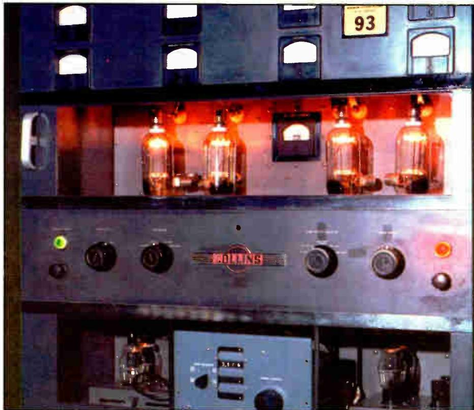
This 1949 Collins 300-G, the original transmitter of WUST(AM) in Washington, is operated by the author. Crystal modules are replaced with a self-contained variable frequency control and RF exciter for operation from 1850 through 7300 kc.
