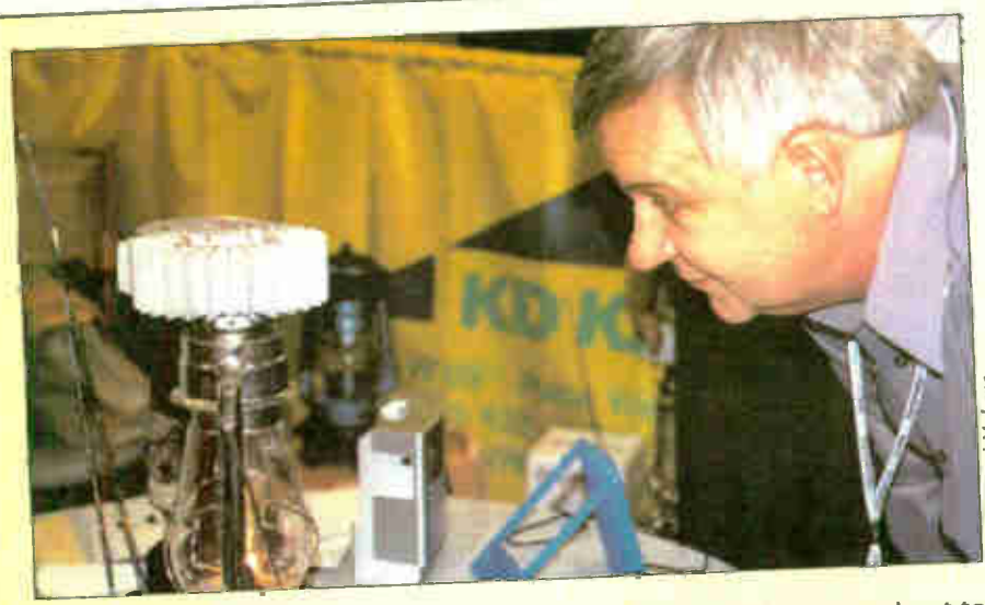
Attendee Dave Biondi inspects the LUFO petrol lamp, which uses heat to generate power for its AM/FM and satellite receiving capabilities. It's aimed at third-world countries and outdoor recreation users.
