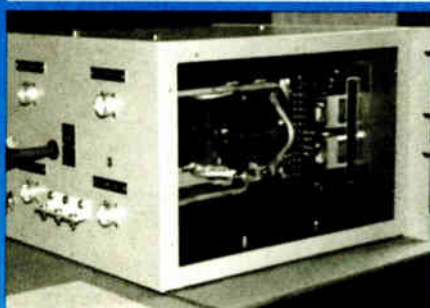
RACK MOUNTABLE MAIN/AUX/DUMMY LOAD TRANSFER SWITCHES
