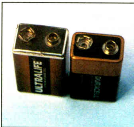
Not all 9V batteries are the same size, and may not fit in battery compartments
