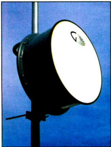
The HSSP(\*)-23 and HSSP(\*)-52 Gabriel antennas are available in 2- to 8-foot diameters and feature plane-polarized feed assemblies with Type N connectors. They deliver high gain and aggressive front-to-back ratios.
