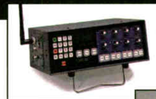
SRPT-40 Frequency agile remote transmitter available in VHF and UHF models
