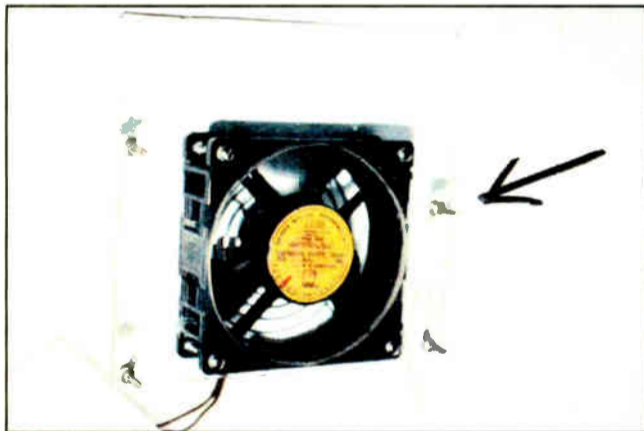
Figure 3: After mounting the fan to the new cover, in this case a piece of Plexiglas, four banana plug jacks are installed for easy mounting to the support rods.
