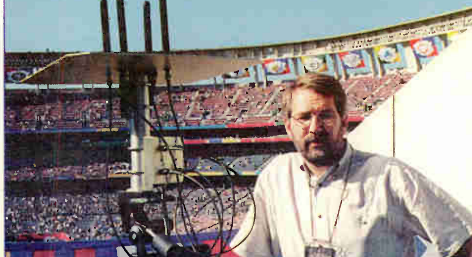
Mike Tosch stands next to one of three DF antenna arrays used during the Super Bowl at San Diego's Qualcomm Stadium.
