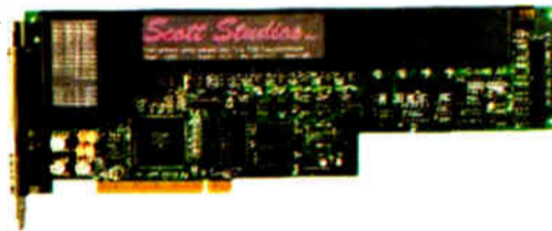
Scott Studios exclusive new 32-bit PCI audio card plays up to four CD quality uncompressed stereo channels while recording!
