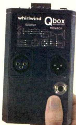
The SPEAKER selector toggles between the SOURCE selections and letting you confirm mic or line level signals from the console.
