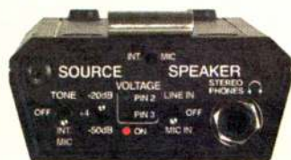
The SPEAKER selector toggles between the SOURCE selections and letting you confirm mic or line level signals from the console.
