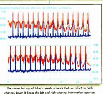
channel. Layer III keeps the left and right channel information separate, maintaining the integrity of the steres signal. Since perception of stereo is in the higher frequencies, Zephyr yields improved stereo perception.
