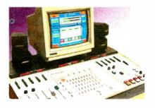
hardened aluminum panels, polycarbonate module overlays, and solid oak trim will provide a durable and attractive appearance through the years.
