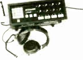
Technology & convenience combine to bring you on-the-spot remote broadcast capabilities with excellent sound quality. Cellular transceiver, frequency extender, and mixer all in one! Powered by Ni-cad rechargeable batteries or AC power supply — utilizes cellular technology or land lines.
