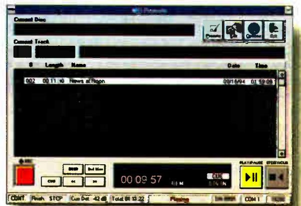
Denon's MD Remote™ Software, running under Windows™, offers a graphical interface for fast, easy control of all functions and modes on any Denon MD Cart machine, including automatic dubbing of tracks or discs between machines, complete with titles and cue-point information.
