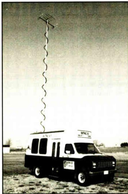
The Will-Burt TMD-7-34 pneumatic telescoping mast extends to a height of 34 feet in seven sections.
