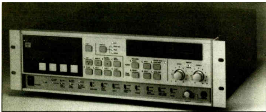
DAT recorders, like this Fostex model, record digital signals on tape by pulse code modulation in a helical scan.
