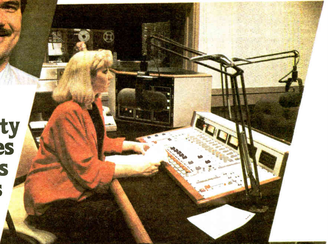
News caster Dawn Matthews on the Audi- tronics 212 in WHIO-AM news studio.
