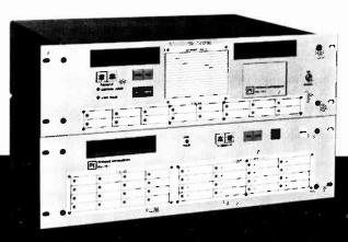
plus 16 status channels. The automatic functions — pattern shift, transmitter restart, power control — are preprogrammed in accordance with station license requirements and controlled with an accurate master clock.
