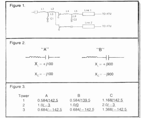
In any array, we would endeavor to keep the network phase shifts close to 90°. Overall system phasing is determined by tower spacing, transmission line length and velocity factor, ATU and network phase shift and power divider phase shift.
