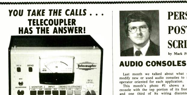
The Telecoupler is designed to interface the telephone to an audio console during two-way conversation such as telephone interviews, telephone talk shows or "on-the-spot" news coverage.
