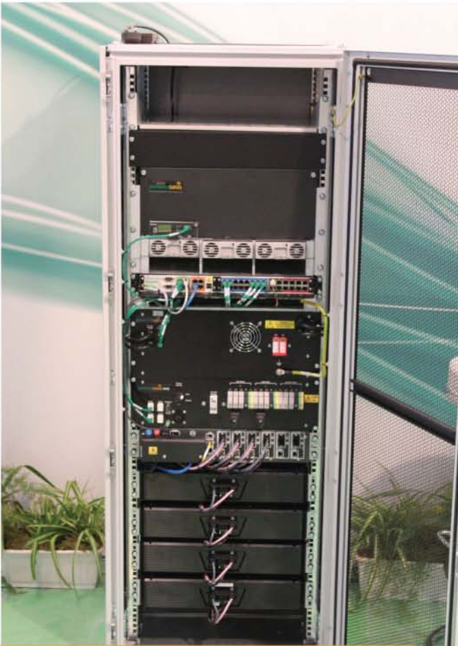
This is the Panasonic Eco Solutions Green Tower comprehensive energy solution for cellular tower and Wi-Fi hotspot sites on display at the Mobile World Congress conducted in March in Barcelona, Spain. The product combines Panasonic's lithium-ion and solar technology expertise with PowerOasis' energy management platform.
