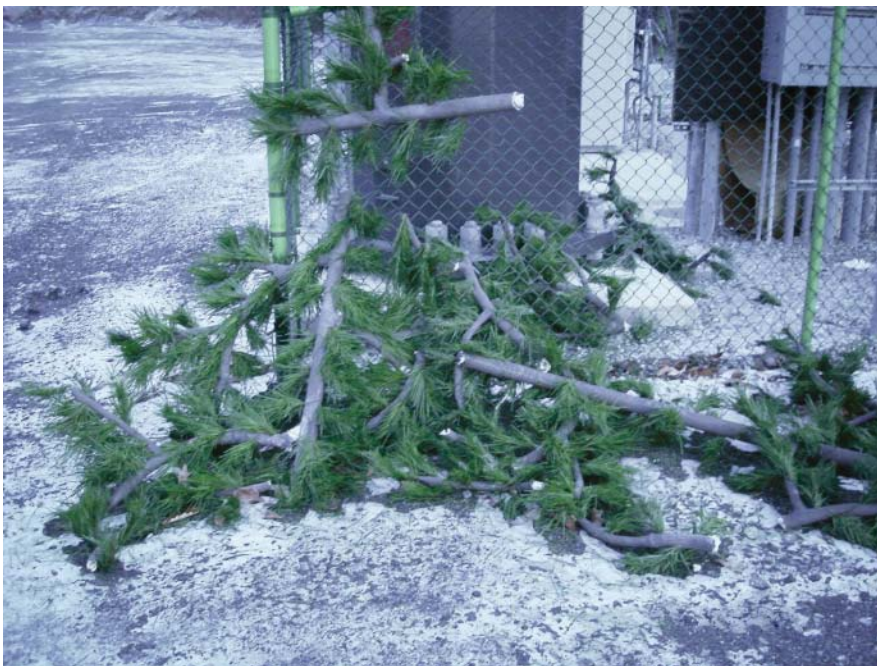
These are from the second set of branches described in the article text on this page. PVC becomes brittle over time — especially in the cold — and has no structural strength of its own. Without a formal structural layup, hand-applied fiberglass mat or roving also has no structural strength of its own.
