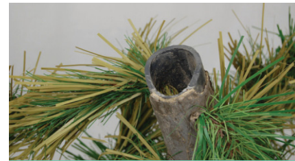
With some manufacturers, the use of solid-cast branches lost ground to brittle plastic tubing that breaks easily when there is little structural support.
