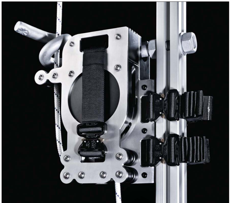
The concept of lead climbing (common in the rock climbing world) linked with using an autolocking pulley on specially designed pig-tail step bolts gave Gegen Absturz the idea for creating the Orca, the world's first industrial lead climbing system with a fully automated braking system capable of taking fall factor two loads within peak loads required by the American National Standards Institute (ANSI) and other international standards.
