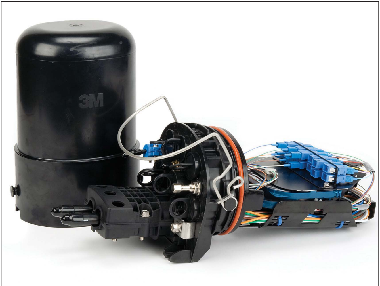
Photo 3. The 3M fiber dome terminal enclosure allows quick and easy connection of the RRU fiber jumper to the tower fiber cabling in a trunked-fiber tower architecture.
