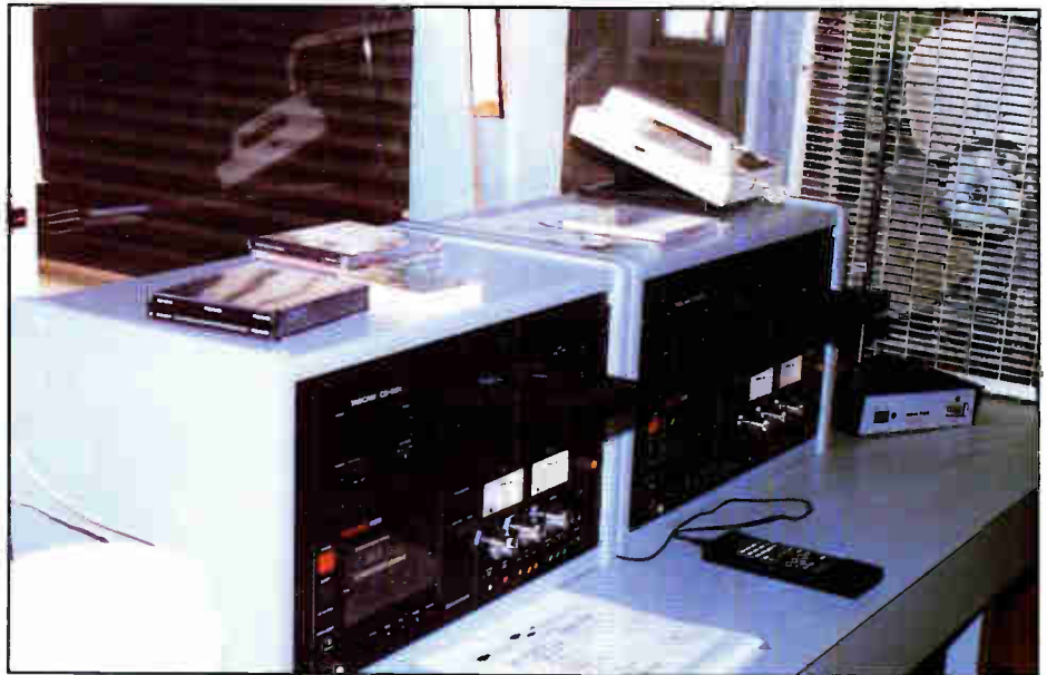
The main control room contains two Tascam CD players to play back the custom zoo CDs. Two cassette decks were included for experimenting with program material.
