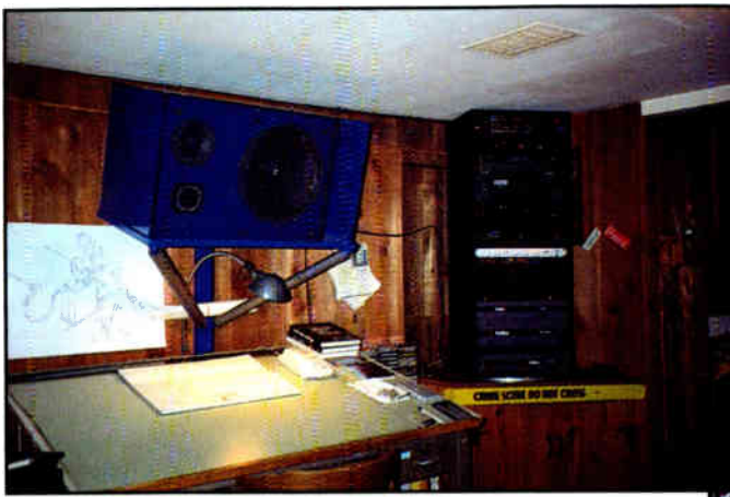
The MAS-486 — a full-range cabinet — is one of five speakers driven by three Hafler Pro series amplifiers at "The Residence."
