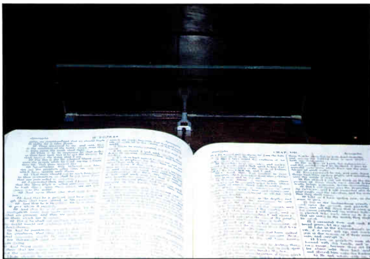
A Crown PZM-6FS mounted to a Plexiglas wedge boundary gives a gradual-proximity effect in "The Church."
