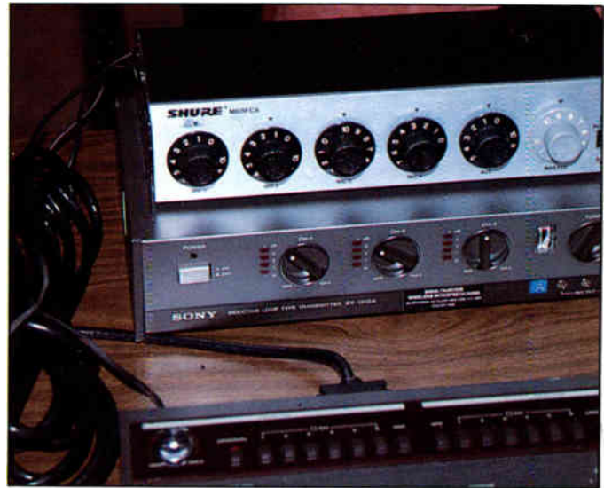
Equipment used in SWI installations: The Sony SX5000B control unit for conference systems (left). The Shure M-68FC 4-channel mixer and the Sony wireless transmitter, the SX-1310.
