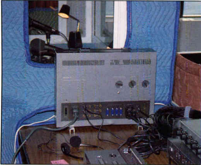
Equipment used in SWI installations: The Sony SX5000B control unit for conference systems (left). The Shure M-68FC 4-channel mixer and the Sony wireless transmitter, the SX-1310.
