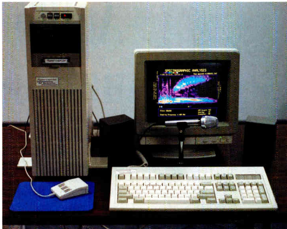
PC-based workstation; note color spectrogram on monitor.
